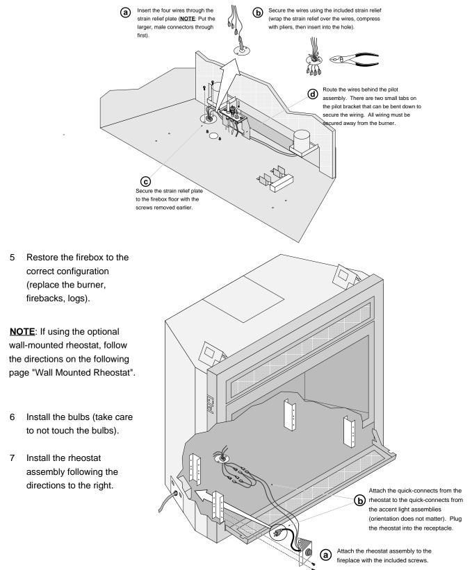
4 Install the strain relief plate to the firebox floor following the directions below.
