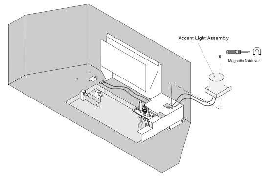
4 Install the remaining accent light assembly to the left burner support. Place the burner support near its original location (do not attach at this time).
