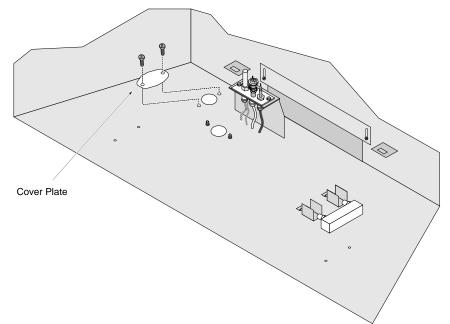
3 Place the rear fireback in position and install the accent light assemblies following the directions below.
